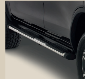
OVAL- STAINLESS STEEL AND MILD STEEL COMBINATION PART NUMBER: PZN68D507
